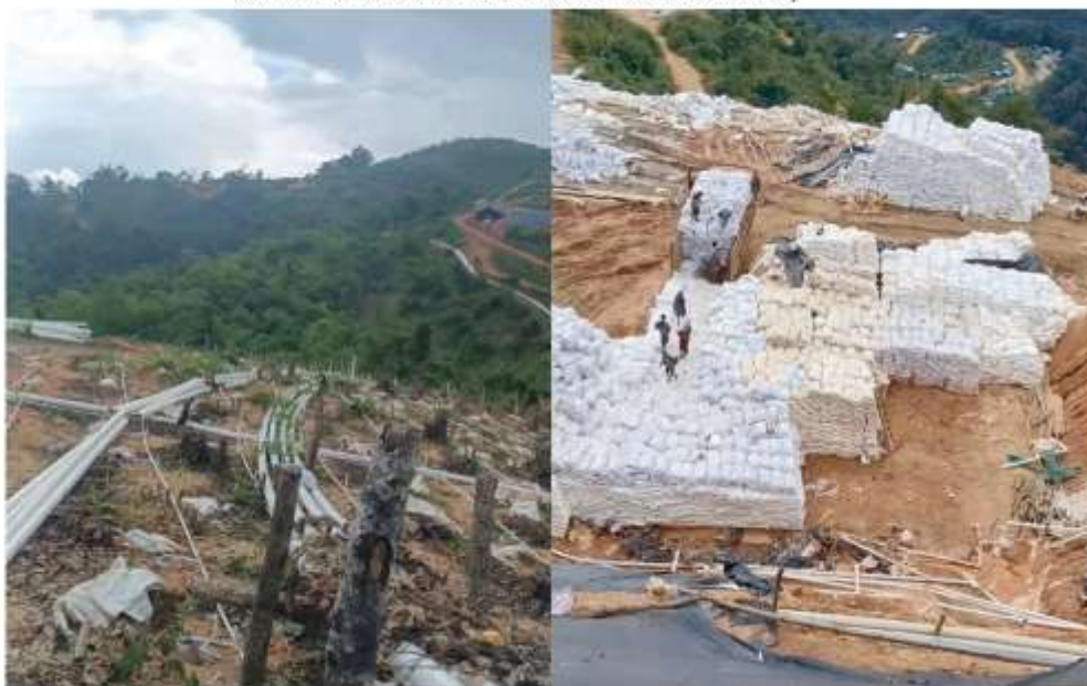
Pipes used for injection of leaching chemicals into mountainside
